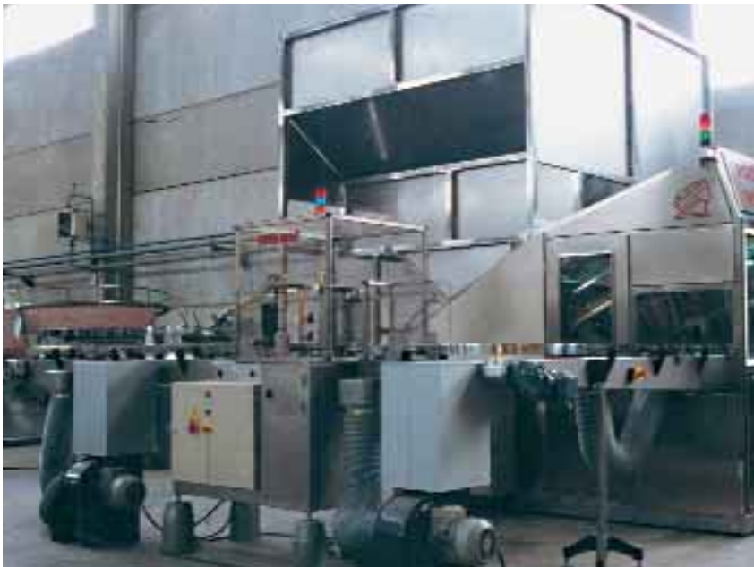
Silo Posisilo, Posimat unscrambler and Giramat orientor
